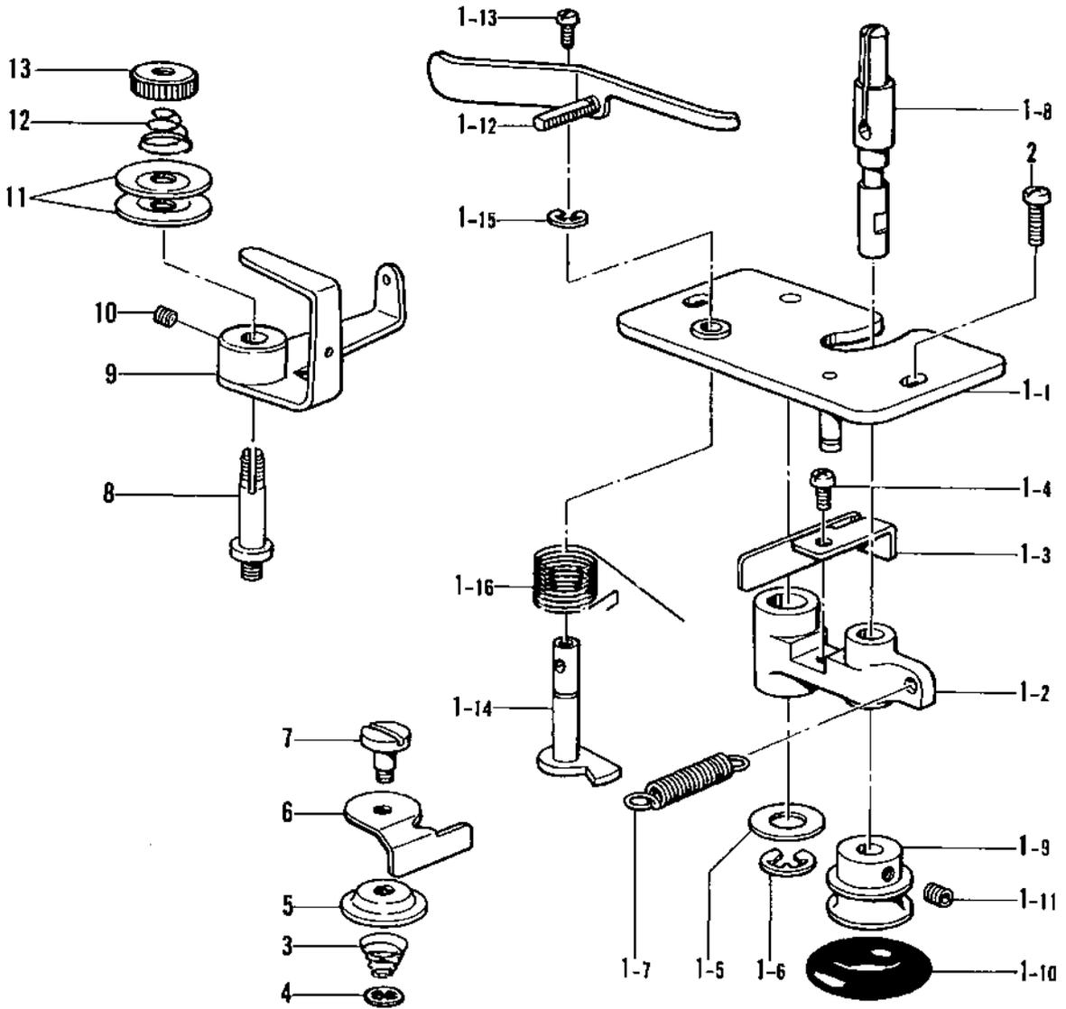
J. 糸巻関係/Bobbin winder mechanism/Spuler/
