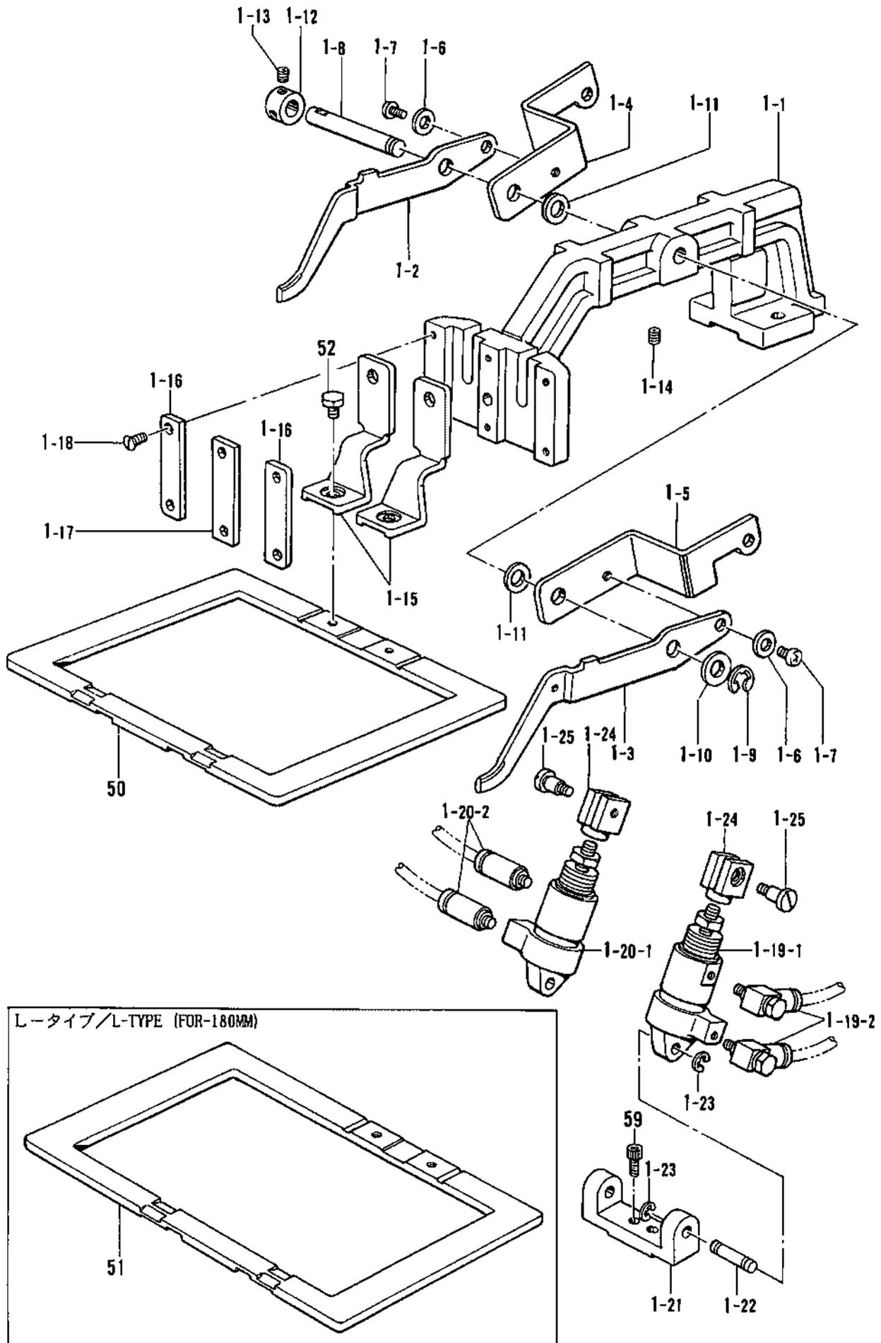
C. 送り関係/Feed mechanism/Transportvorrichtung/
