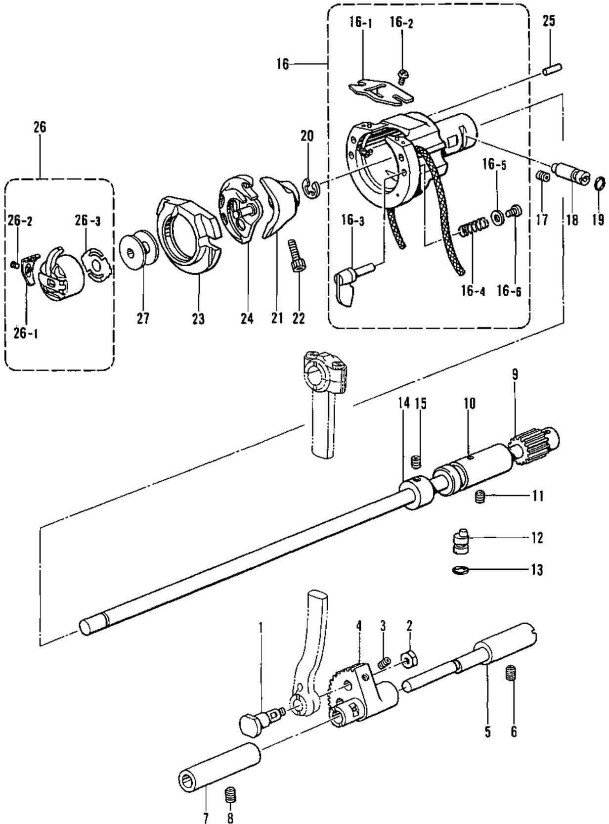
F. 下軸関係 / Lower shaft mechanism / Untere Welle /
