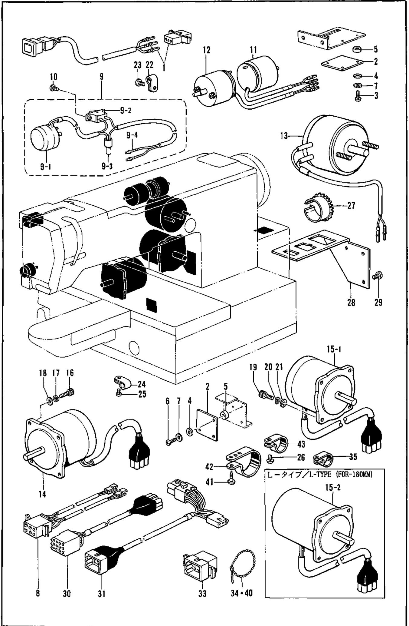
N. 電装品関係 / Power supply equipment mechanism / Stromversorgung /
